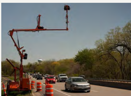
Acusensus Heads-Up Real Time solution detects passing vehicles.
